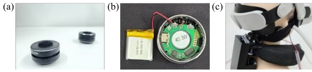
Figure 6: (a) BCV device used in this experiment, (b) inside of the BCV stimulator, and (c) device attached to the participant.
