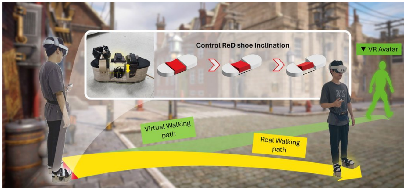
Fig. 1 Conceptual illustration of the ReD Shoes in action, demonstrating the control of shoe inclination to enable redirected walking in a virtual environment
