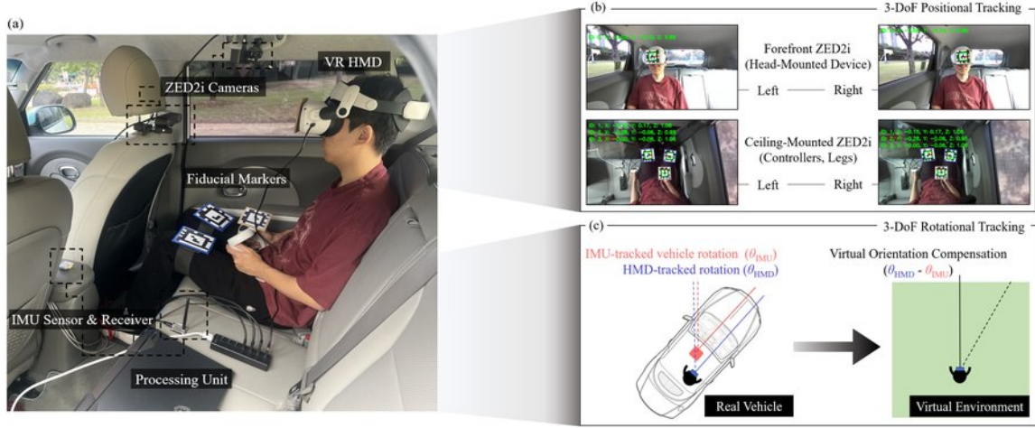
Figure 2: (a) 6-DoF tracking setup in the passenger seat of a vehicle, with an integrated tracking platform. (b) Visualization of fiducial marker detection between the two ZED2i cameras, translated into position tracking within VR. (c) Explanation of the compensation method utilized by the IMU sensor fixed to the vehicle for headset rotation tracking.
