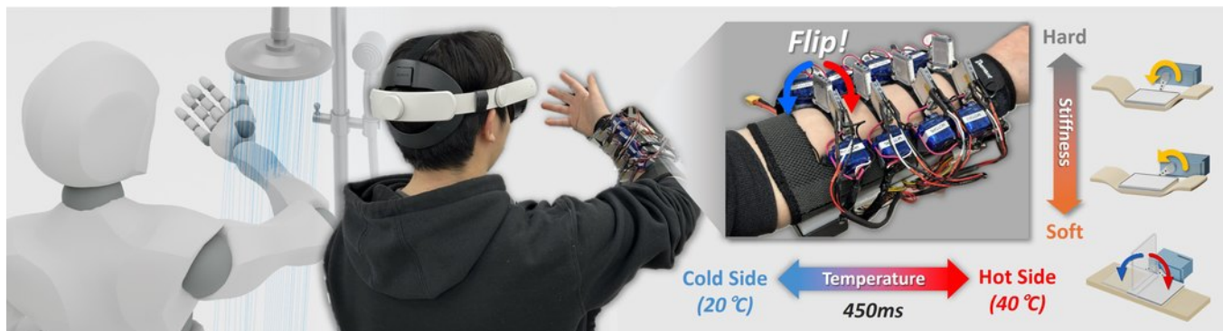
Figure 1: The Flip-Pelt system showcases a motor-driven peltier element concept, utilizing the dual-sided functionality of pre-heated or cooled elements and enabling rapid thermal transitions with a 450ms motor operation speed. Moreover, this design simulates the stiffness of contact materials through congruent pressure feedback alongside thermal sensations.
